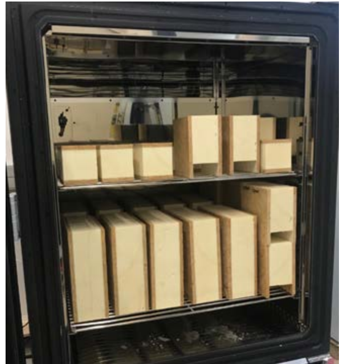
Small-scale SIP samples in climate chambers for accelerated ageing
